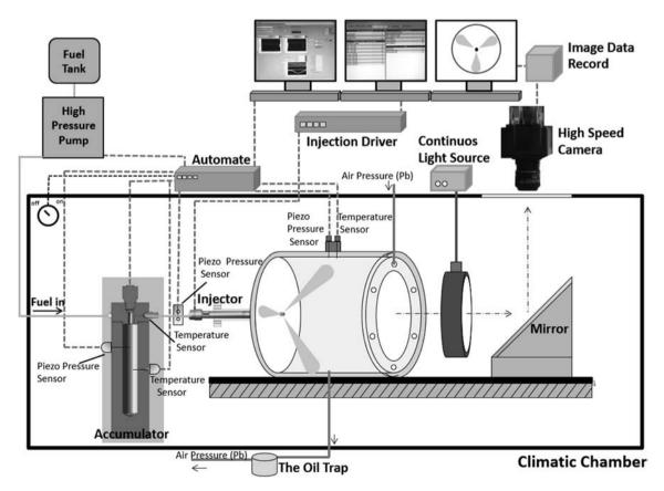
Fig. 2. Experimental setup for spray injection.
