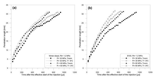
Fig. 12. Mean penetration length on the 3 sprays -Pi = 30, 60 MPa, Pb = 1.2 MPa when (a) winter diesel and (b) B100.
