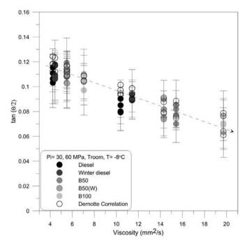
**Fig. 16.** The average spray angle versus viscosity, experimental data and Dernotte correlation -Pi = 30, 60 MPa.
