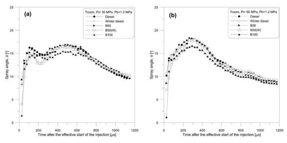
Fig. 14. The spray angle -Troom at (a) Pi = 30 MPa and (b) Pi = 60 MPa.
