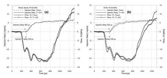
Fig. 6. Mean mass flow rate and Pline - Pi, Pi = 30 MPa when (a) winter diesel and (b) B100.
