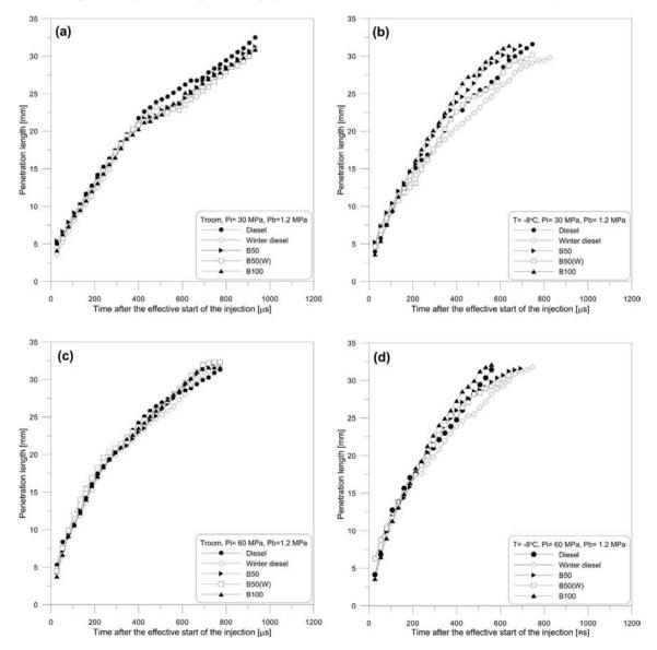
**Fig. 13.** Mean penetration length all fuel at (a) Troom, Pi = 30 MPa, Pb = 1.2 MPa, (b) T =  $-8 \degree C$ , Pi = 30 MPa, Pb = 1.2 MPa, (c) Troom, Pi = 60 MPa, Pb = 1.2 MPa and (d) T =  $-8 \degree C$ , Pi = 60 MPa, Pb = 1.2 MPa.
