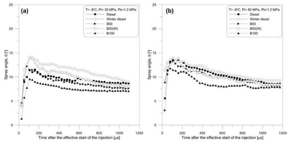
**Fig. 15.** The spray angle  $-T = -8 \degree C$  at (a) Pi = 30 MPa and (b) Pi = 60 MPa.
