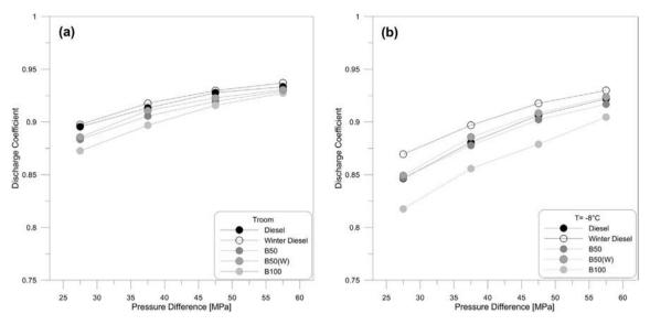
Fig. 7. Impact of fuel blends and temperature on the discharge coefficient -Pi = 30-60 MPa at (a) Troom and (b) T = -8 °C.
