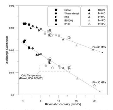
Fig. 9. Impact of fuel kinematic viscosity on the discharge coefficient - Pi = 30, 60 MPa, T = Troom, 8 °C, -5 °C and -8 °C.
