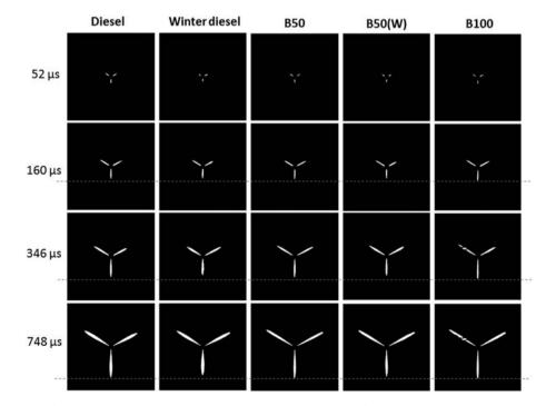
Fig. 11. Comparison of spray development: average image 52 µs, 160 µs, 346 µs and 748 µs after injection – T = –8 °C, Pi = 30 MPa, Pb = 1.2 MPa.
