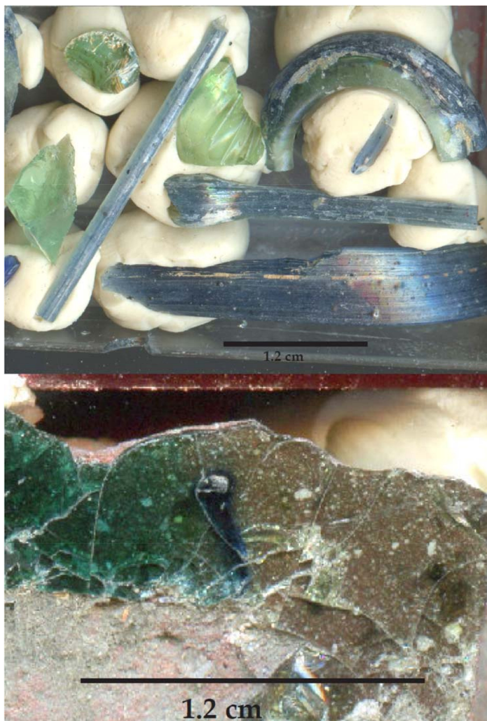
Figure 1. Cobalt colourant inclusions in the glass waste from Beirut ( upper ) and the crucible from Grozon ( bottom ). For Beirut several black inclusions the sizes of which range from some tens to some hundreds of micrometers were analysed, while for Grozon several analytical points were done on and around a larger inclusion which is approximate about 1 mm in diameter.
