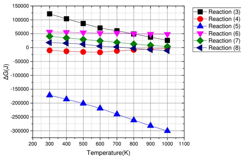
**Figure 5.** Gibbs energy as a function of the temperature for reactions (3) to (8) (calculated using CIRCE code under 80 bar pressure).
