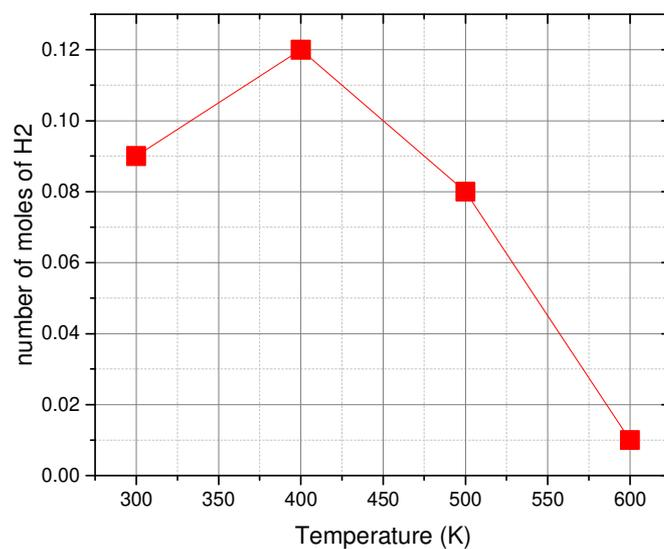
**Figure 6.** Calculated evolution of the maximum number of H<sub>2</sub> moles produced during the heating up of the vessel (CIRCE code: 55 g water, 6 g carbon in a 100 ml volume).
