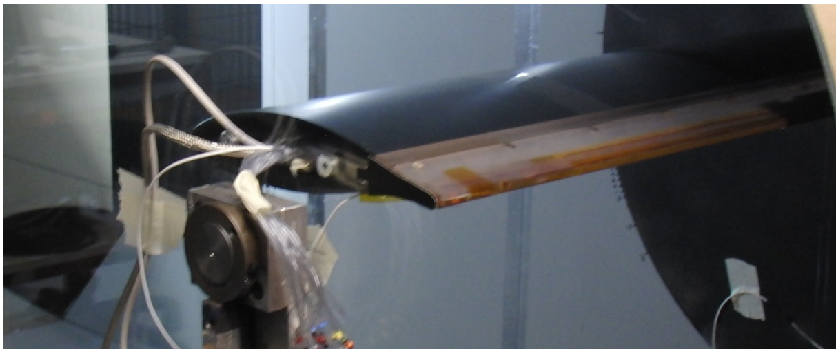
Figure 6. Photography of the airfoil model mounted on the wind tunnel test section
