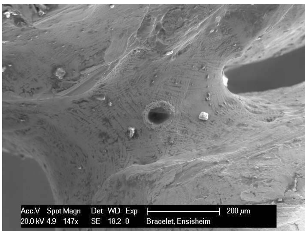
Figure 1. SEM images of laser ablation craters made on prehistoric gold artefacts using the two laser equipment available in the IRAMAT-CEB: (a) Nd:YAG; (b) ArF-excimer. © CNRS IRAMAT-CEB
