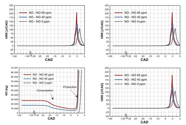
Figure 46. CFD computed heat release traces and NO in-cylinder mass traces as a function of the initial NO concentration and for two different operating conditions: SOI = -50 CAD and SOI = -20 CAD. Initial conditions are reported in **Table 5**.
