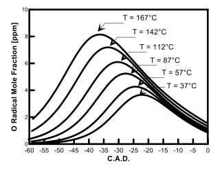
Figure 104. In-cylinder O atoms mole fraction as a function of the CAD for different intake temperatures for an intake Ozone concentration of 100ppm.
