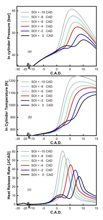
Figure 117.In-Cylinder Pressure (a), In-Cylinder Temperature (b) and Heat Release Rate (c) as a function of CAD for different SOI2.
