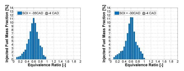
Figure 60. CFD computed fuel distribution as a function of the equivalence ratio for two injection timings corresponding to a spray target position in the lower bowl region. Initial conditions are reported in Table 7
