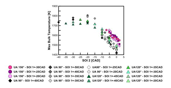
Figure 67. In-cylinder maximum bulk temperature as a function of the SOI1 and SOI2 and for different injector umbrella angles. Experimental conditions are reported in Table 7
