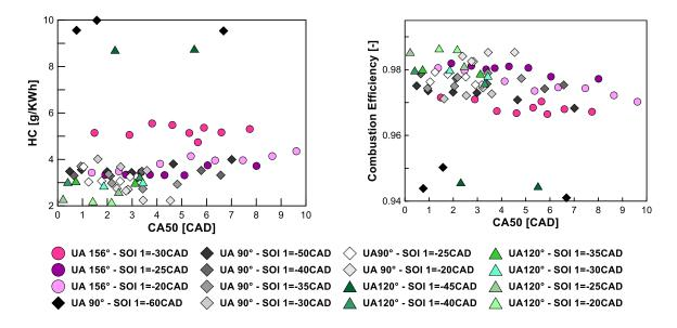
Figure 71. HC emission and combustion efficiency as a function of CA50 and for different injector umbrella angles. Experimental conditions are reported in Table 7
