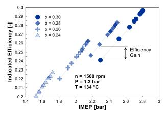
Figure 88. Indicated efficiency as a function of IMEP for different values of the fuel-air equivalence ratio.
