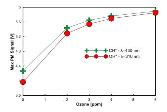
Figure 97. Impact of ozone concentration in ppm on the maximum intensity of the signal of CH\* and OH\* measured by photomultipliers. Experimental conditions are reported in Table 12.
