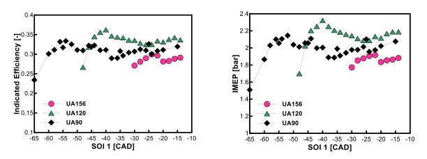
Figure 55. Experimental indicated efficiency and IMEP as a function of SOI and for the different umbrella angles. Experimental conditions are reported in Table 7
