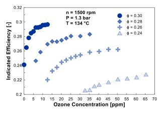
Figure 87. Indicated efficiency as a function of intake ozone concentration and for different fuel-air equivalence ratios.
