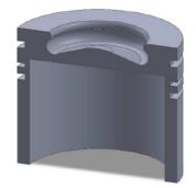
Figure 19. Vertical section of the piston in the DW-10 engine
