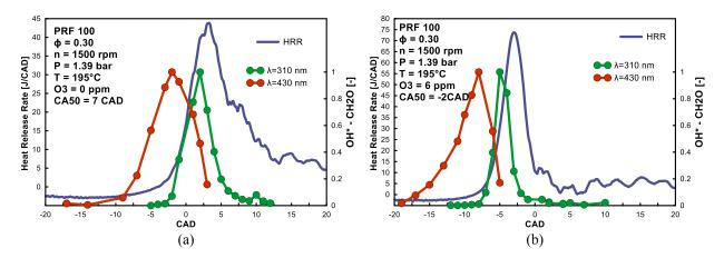
Figure 95. Impact of ozone addition on the heat release rate, CH2O and OH\* integrated signal for thermodynamically induced combustion. Heat release, OH\* and CH<sub>2</sub>O are reported for the non-seeded case (a) and for the seeded case with the ozonizer capacity set to 4%, corresponding to 6 ppm of O<sub>3</sub>. (b). Experimental conditions are reported in Table 12.
