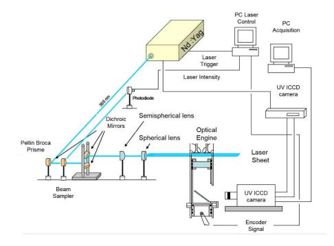
Figure 24. Schematic of the CH<sub>2</sub>O PLIF acquisition system.
