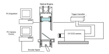
Figure 22. Schematic of the OH\* chemiluminescence acquisition system.
