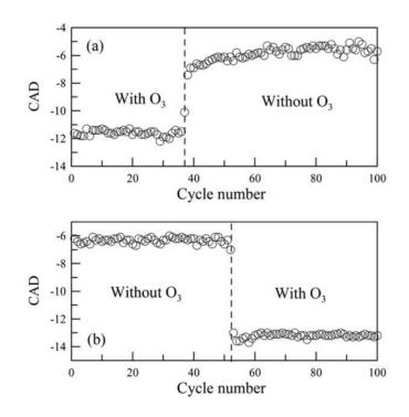
Figure 13. Variation of the phasing of the main flame induced by switching on and off the ozone generator. (a) Direct case off – on. (b) Reverse case off-on. From [85]
