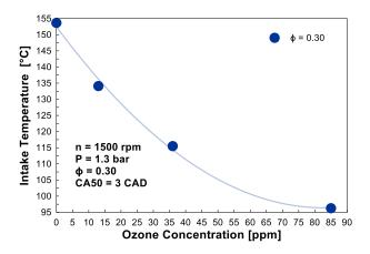
Figure 89. Intake temperature required to achieve combustion by placing the CA50 3 DA after TDC, as a function of the intake ozone concentration.
