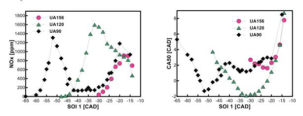
Figure 56 reports the NOx emission and the combustion phasing CA50 as a function of the SOI, for the three injectors tested.
