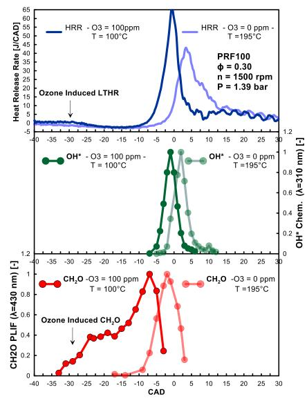
Figure 99. Heat release rate trace, OH\* and CH<sub>2</sub>O PLIF emission under TI and OI conditions. Experimental conditions are reported in Table 13.
