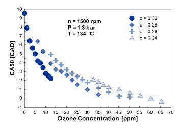
Figure 83. CA50 as a function of intake ozone concentration for different values of the equivalence ratio of the fuel-air mixture.
