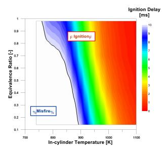
Figure 33. Constant volume ignition delay calculation for a gasoline surrogate fuel [117] as a function of equivalence ratio and temperature for a constant initial pressure of 32 bar.
