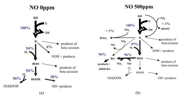
Figure 17. Flow analysis for the stoichiometric oxidation of 1500 ppm of n-heptane in a PSR at a pressure of 10 atm and a temperature of 665 K with addition of (a) 0 ppm of NO and (b) 500 ppm of NO. Adapted from [106].
