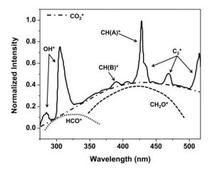
Figure 23. Chemiluminescence emission of OH\*, CO<sub>2</sub>\*, HCO\*, CH2O\*. From [109]
