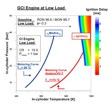
Figure 31. Schematic representation of the autoignition process inside a GCI engine at low load.
