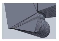
Figure 27. The CFD computational domain was built from the geometry of the customized DW-10 engine piston
