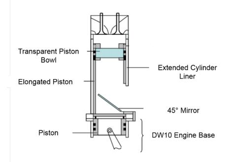
Figure 20. Schematic representation of the optically accessible engine.
