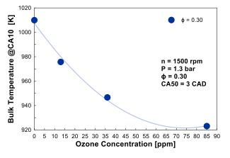
Figure 90. Intake temperature required to achieve combustion by placing the CA50 3 DA after TDC, as a function of the intake ozone concentration.
