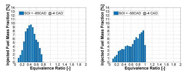
Figure 58. CFD computed fuel distribution as a function of the equivalence ratio for two injection timings corresponding to a spray target position in the upper bowl region. Initial conditions are reported in Table 7
