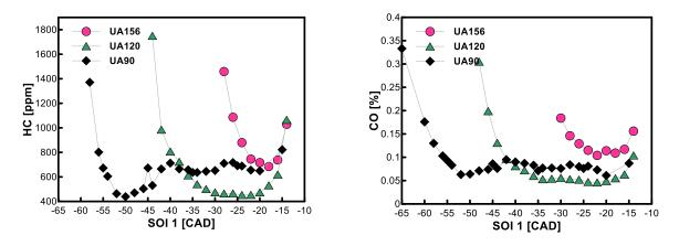
Figure 52. HC and CO exhaust concentration as a function of SOI and for the different umbrella angles. Experimental conditions are reported in Table 7 mechanism which determined the ability of the narrower umbrella angle to extend the high combustion efficiency SOI range.
