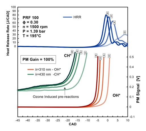
Figure 98. Heat Release Rate (HRR) traces, OH\* and CH\* signals from photomultipliers as a function of different ozone concentrations. Numbers in the boxes indicate the ozone concentration in ppm. Photomultiplier gain was set at full capacity. Experimental conditions are reported in Table 12.
