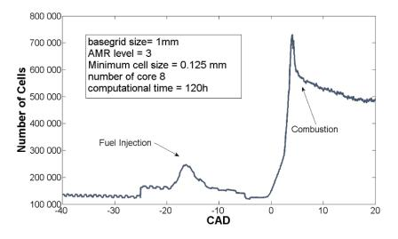
Figure 29. Cell count during the simulation of the engine cycle.
