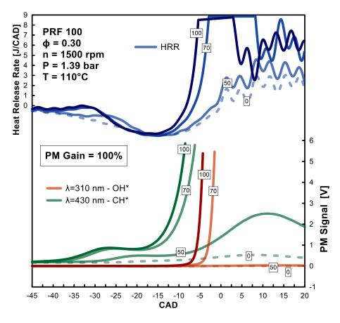
Figure 101. Impact of ozone addition on the heat release rate, OH\* and CH\* signals from photomultipliers. Numbers in the boxes indicate the ozone concentration in ppm. Photomultiplier gain at 100%. Experimental conditions are reported in Table 12.
