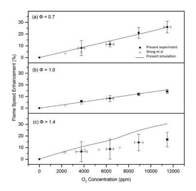
Figure 10. Promoting effect of ozone on the laminar flame speed of  $CH_4$ . P = 1 bar and T= 300 K. Adapted from [81]
