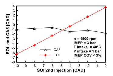
Figure 116. End of Injection and CA10 as a function of the SOI2
