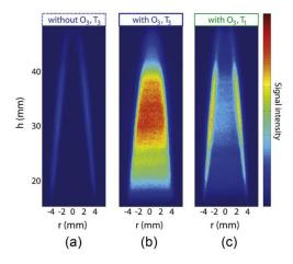
Figure 11. CH<sub>2</sub>O production enhancement induced by ozone. From [76]
