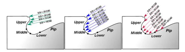
Figure 51. Spray target position as a function of the SOI different umbrella angles. A second drop in combustion efficiency delimited the earlier admitted SOI, whose position was instead
