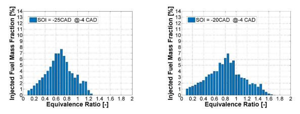
Figure 61. CFD computed fuel distribution as a function of the equivalence ratio for two injection timings corresponding to a spray target position in the lower bowl region. Initial conditions are reported in Table 7
