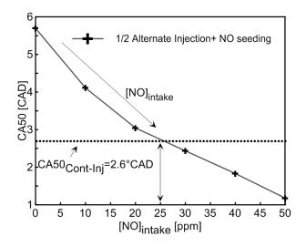
Figure 43. Experimental evaluation of the NO trapped fraction. CA50 as a function of NO concentration, during alternate-fired mode. Experimental conditions are reported in **Table 5**, but intake temperature was reduced to  $T = 175^{\circ}C$ .
