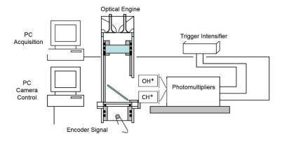
Figure 26. Schematic of the simultaneous OH\* and CH\* chemiluminescence acquisition system by means of a double detector photomultiplier.
