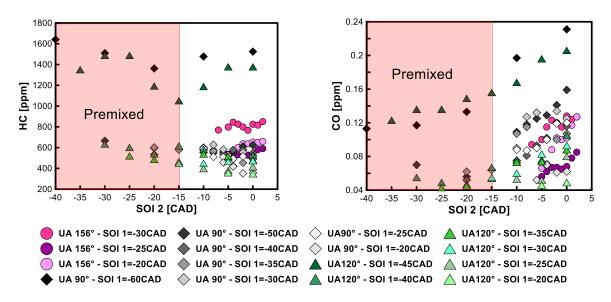
Figure 66. HC and CO as a function of SOI1 and SOI2. Experimental conditions are reported in Table 7
