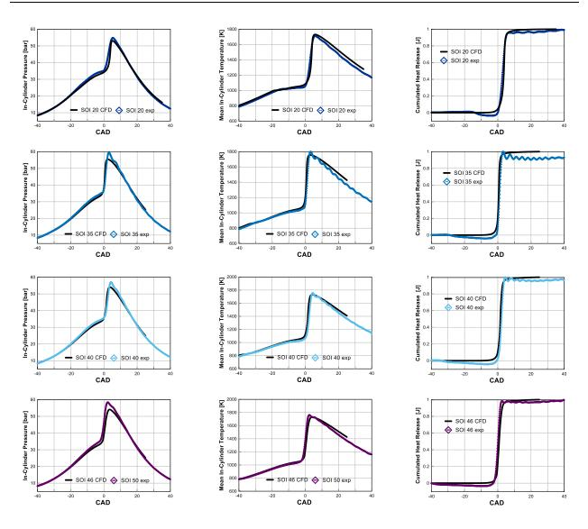
Figure 30. Experimental and calculated in-cylinder pressure, temperature and normalized cumulated heat release rate as a function of the injection timing.
