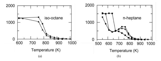
Figure 16. Impact of NO addition on iso-octane (a) and n-heptane (b) oxidation, adapted from [105]. Figures show the Species concentration profiles during the stoichiometric oxidation of n-heptane in a jet-stirred reactor at 10 atm with a residence time of 1 s in the presence of various amounts of NO: 0 ppmv (circles), 50 ppmv (triangles), 500 ppmv (squares).
