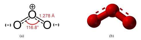
Figure 9. Skeletal formula of ozone (a). Ball and stick model of the Ozone molecule (b).
