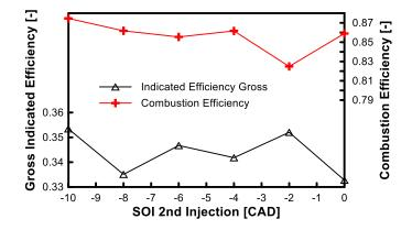
Figure 119. Combustion Efficiency and Gross Indicated Efficiency as a function of the SOI2.
