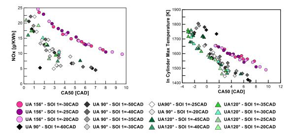
Figure 69. NOx emission and maximum bulk temperature as a function of CA50 and for different injector umbrella angles. Experimental conditions are reported in Table 7
