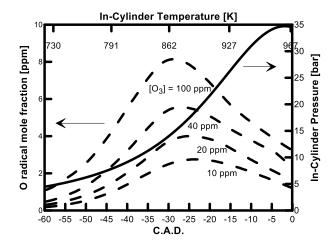
Figure 103. O atoms mole fraction and in-cylinder pressure as a function of CAD for different ozone concentrations at the intake. ozone despite the recombination of O atoms into O<sub>2</sub> molecules. The final purpose of the use of ozone is to systematically reduce the intake air temperature required for low load gasoline autoignition.
