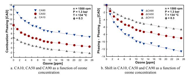
Figure 75. Impact of different ozone concentrations on the phasing of HCCI combustion of gasoline 5.3.1.1.Impact on the combustion phasing
